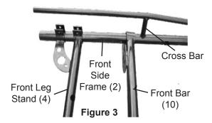
For Long Bed Truck (7' or more): Slide Front Bar (10) onto FRONT ends of Front Side Frames (2). Then slide Front Leg Stands (4) onto Front Side Frames so they are in front of Frame's cross bar. See Figure 4, below.
